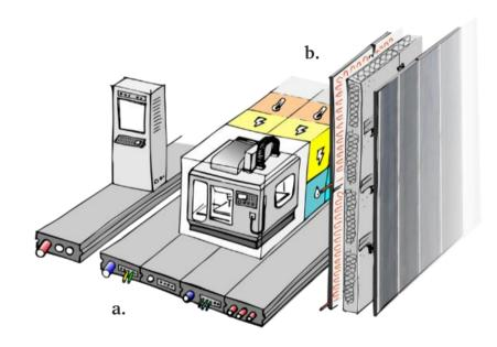
Example drawing: a) floor or ceiling module for energyefficient design of energy networks, b) thermally activated wall module
