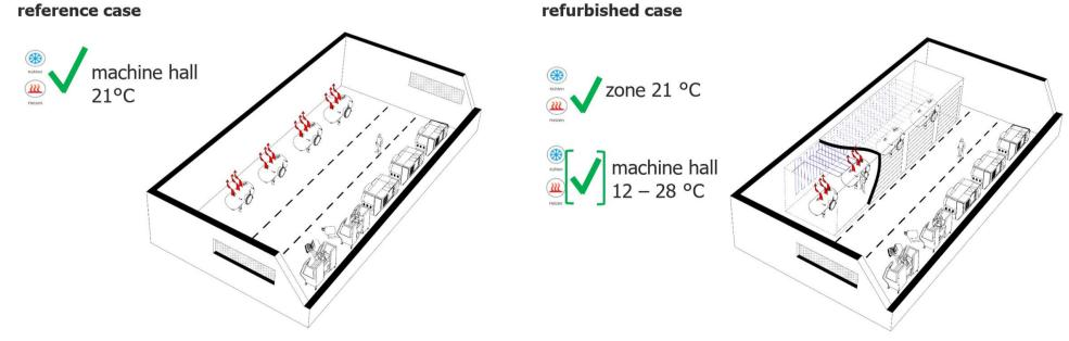
Comparison of a reference factory building and a refurbished factory building with thermal zoning of the machines
