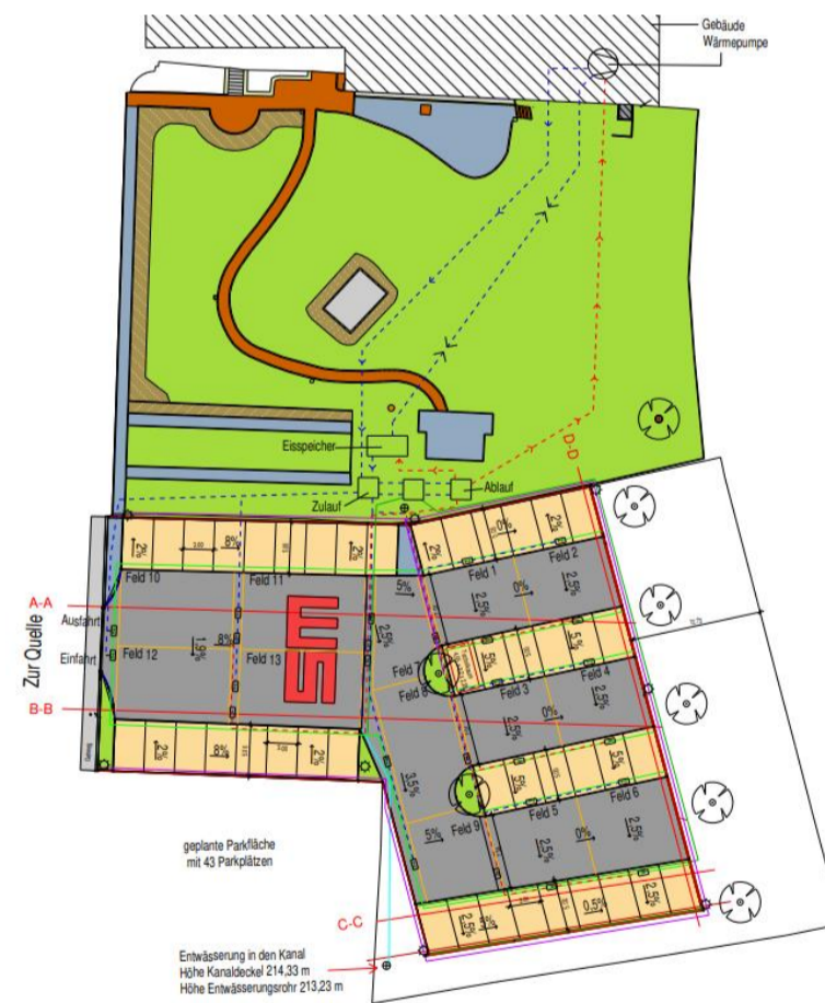
Fig. 2: Site plan and schematic connection concept between the building and asphalt solar collector
