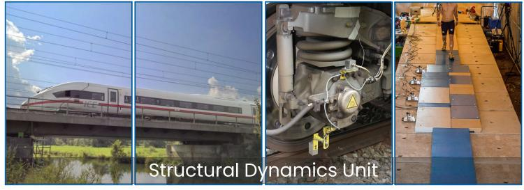
The Structural Dynamics Unit of the Institute of Structural Mechanics and Design deals with a series of projects that investigate vibrations on bridges and their effect on the structure's service life prediction. Moreover, the respective impact of
